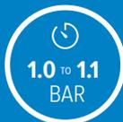
The system pressure should be set around **1.0 – 1.1 bar** when the water is cold.
