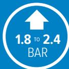
When the system is working and the water is heated up within the system, water expands due to heat and you may see the pressure rise up to around **1.8 – 2.4 bar** when hot. This is normal as water system pressure increases due to heat. So we are looking for the system pressure to be set around **1.0 – 1.1 bar** when the water is cold.
