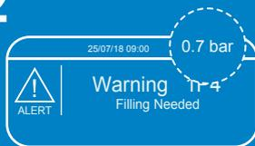
The pressure within the system can be seen in the top right of the display when an error code comes up.
