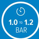
The system pressure should be set around **1.0 – 1.2 bar** when the water is cold.
