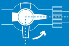
The taps should be **opened a quarter of a turn** and the water will start to refill the system (water should be heard filling the system). You should see the pressure gauge rise back up between 1 bar and 1.2 bar pressure and then stop filling. The error code 118 will stop and the boiler will now operate. If the error code 118 is still active, fill up the system a little more but **NOT** over 1.4 bar.
