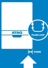
On the iC and iC Economiser Plus models, to re-pressurise the system you will need to **find the filling loop** (copper 'U' shaped tube with two nuts at each end). On the underside of the boiler there is a filling loop position where this copper 'U' shaped tube will connect between the small blue and black isolation valve connection (iS boilers have an external filling loop on the system). If not in position, remove the caps and install as shown and tighten up the nuts hand tight.
