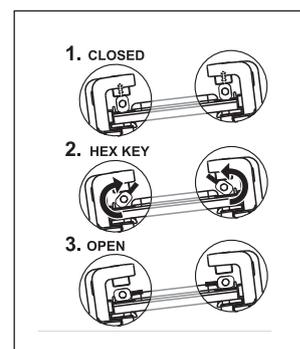
**The following operations must be performed carefully in relation to the vulnerability of the non return valve.**
