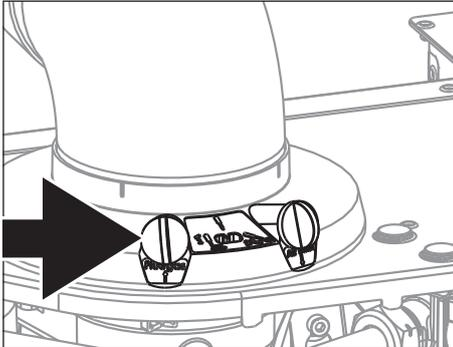
The CO<sub>2</sub> percentage is set in the factory. This has to be checked during commissioning, inspection, maintenance and in case of a failure.
