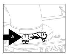
Measuring point CO<sub>2</sub> Figure 15.1.a
