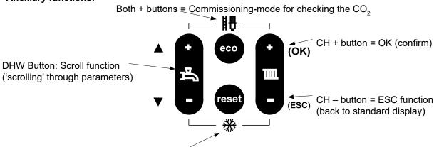
Both - buttons: Pump continuous on/off
