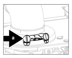
Measuring point CO<sub>2</sub> Figure 15.1.a
