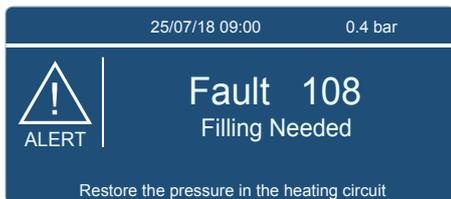
If the water pressure drops below 0.5 bar the text "Fault 108 Filling Needed, Restore the pressure in the heating circuit " will appear in the screen; The air purge program starts when the water pressure has been below 0.5 bar. The automatic air purge program will take approx. 7 minutes and will be followed by the home screen when the water pressure is taken above 1.2 bar.
