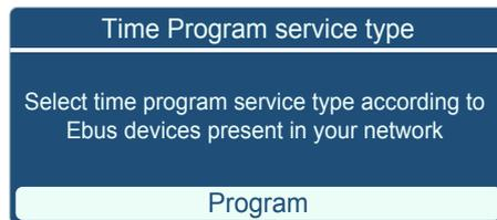
If the time program service type is set from 'Extended Time Program' to 'Program' you will switch from day heating line (contact open) to night heating line (contact closed), which would mean on and off.
