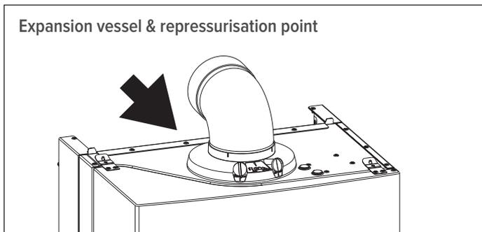
**Note:** The vessel can lose some of its charge pressure over time. Also check whether the installed expansion vessel is adequate for the system water volume.
