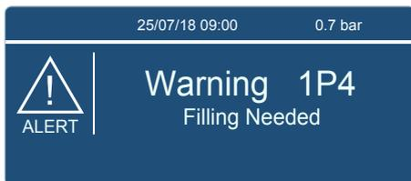
If the water pressure drops below 0.8 bar the text "Warning 1P4 Filling Needed" will appear in the screen;
