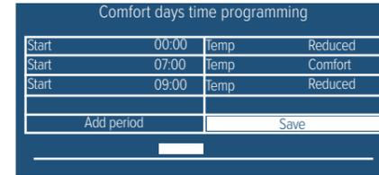
This screen is where you can have the hot water preheat start from 00:00 (midnight) with an off period (shown as Reduced) to the 07:00 where the hot water is set to an on period (shown as Comfort).
