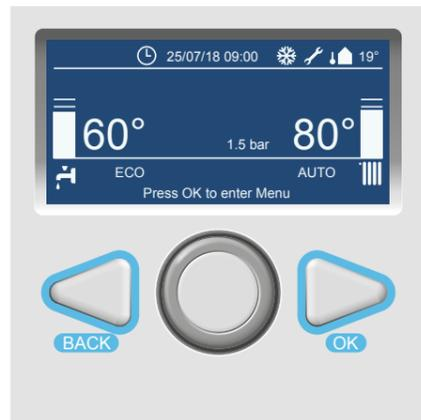
1 From the controller Home screen, press the **BACK** and **OK** buttons at the same time for 7 seconds.
