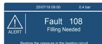
If the water pressure drops below 0.5 bar the text "Fault 108 Filling Needed, Restore the pressure in the heating circuit" will appear in the screen; The air purge program starts when the water pressure has been below 0.5 bar. The automatic air purge program will take approx. 7 minutes and will be followed by the home screen when the water pressure is taken above 1.2 bar.
