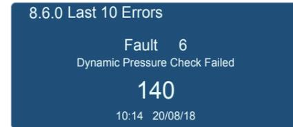
**Error codes** A detected failure is indicated on the display using error messages. Any blocking error, which includes a P (1P4, 1P9 etc), will only be visible using the Last 10 errors function.
