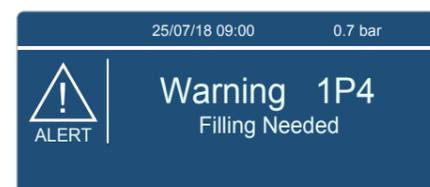
If the water pressure drops below 0.8 bar the text "Warning 1P4 Filling Needed" will appear in the screen; Between 0.5 and 0.8 bar and the boiler will reduce Tset max by 5°C.
